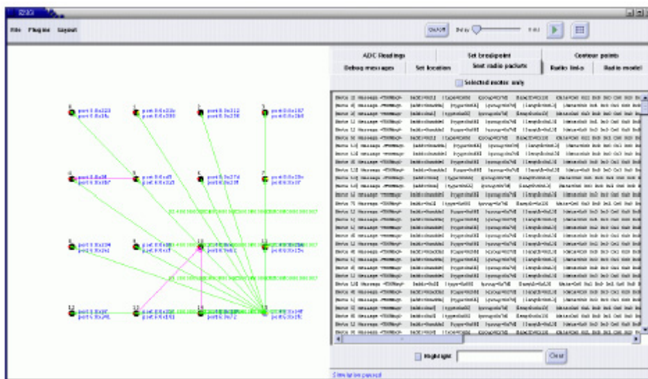
Figure 6. TinyViz connected to TOSSIM running an object tracking application (from [4]).
